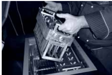
5. Remove one mold at a time and dip in cold water for a few seconds.
