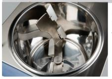
Provided with eccentric blades, the only one without central shaft to mix homogeneously and continuously any ingredient without stressing product texture, especially pastry cream during its cooling and storage.
